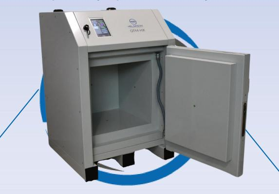
It includes six 45x45x5cm plastic scintillator detectors with PMT and six HV sources. This guarantees that the detectors perform in their optimum operating conditions, providing and excellent signal output.
